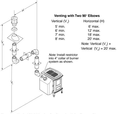
Figure 36 - Vertical Rigid Venting Configuration Using Two 90° Elbows
